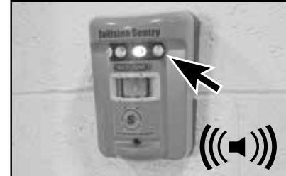
If the Collision Sentry Multi-Zone has detected its pair and motion is detected on both devices, both devices will display the "Motion Detected" blink pattern. Flashing red LEDS and an audio indication.
