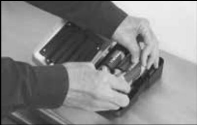
Each Collision Sentry Multi-Zone unit operates on 6 standard D-Cell batteries that are easily replaceable.
