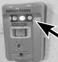
Always activate the units prior to installation. To activate the Multi-Zone, you need to install batteries. Open the Battery Door on one of the units and insert 6 D-Cell batteries in the direction indicated on the battery box. It does not matter which unit is activated first. Once the batteries are installed, the unit goes through a warm-up period of about 35 seconds. Activate the second unit in the same manner with the remaining 6 D-Cell batteries.
