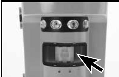
The field of vision on the Multi-Zone is adjustable allowing the area where motion is picked up to be customized for the specific situation. Changing the field of vision is done by adjusting the moveable shades. Each sensor can range from 50 to 134 degrees.
