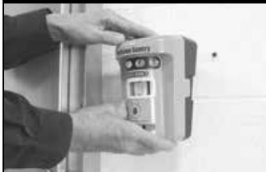
The ideal placement for each unit is at a height between 7' and 9' (2.2-2.75 m). The Collision Sentry Multi-Zone can be magnetically or mechanically attached to walls and other substrates.
